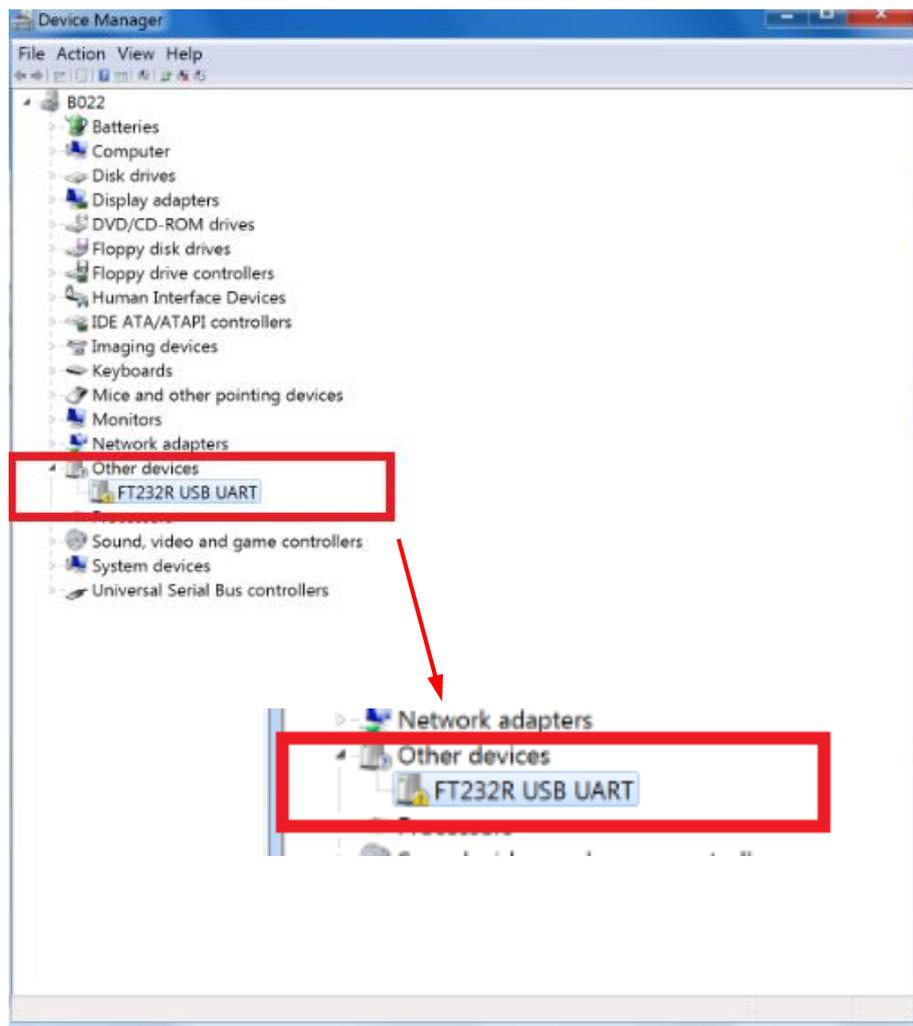
Figure 4. Driver is not installed normally
