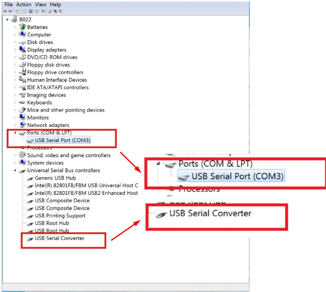
Figure 5. Driver is installed correctly
